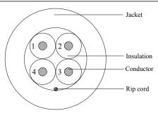
This cable is constructed by cabling together four conductors of 22 awg stranded bare copper conductors insulated with color coded polyvinyl chloride into two pairs, individually shielded. A jacket of gray colored polyvinyl chloride completes
