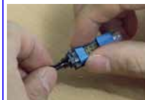
To remove or re-terminate the connector, simple unscrew the boot and replace the jig
