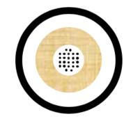
Plenum Multimode OM3 Fiber Cable is constructed with twenty-four internal tight buffers, internal aramid yarn, and one outer riser-rated PVC jacket in distribution format. The fiber cable features a water-resistant jacket and is designed for indoor and outdoor applications.
