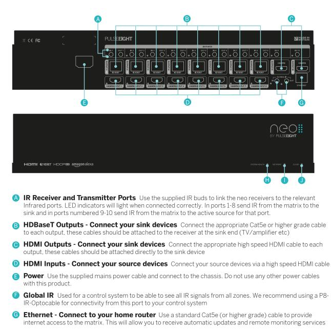
**G** System Health LED Indicator When system is running correctly, the LED will light green
