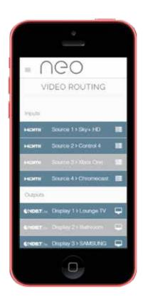
With MatrixOS you can control your matrix from any mobile device that is connected to the same network, simply by visiting www.gotomymatrix.com
