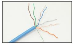
Separate each wire pair by untwisting.
