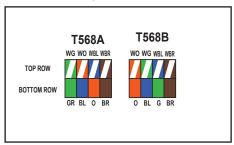
Align wires according to Termination Pattern either Type A or Type B. Hint: Hold wire so that the White Orange and Orange wires are closest to you and put in wire pattern order 1-8.
