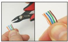
Using a flush cutter, trim the wires straight across so all of the wires are the same length.
