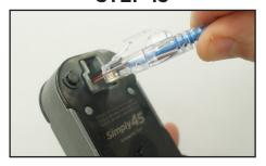
Insert the plug into the crimping socket on the **\$45-C100/\$45-C101** Simply45 pass through crimper.
