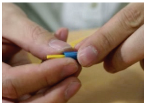
Insert the connector boot and adapter tube onto the cable
