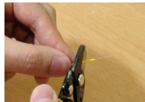
Strip the buffer to the 250μm mark using the middle hole, then the small hole on the stripper in short increments
