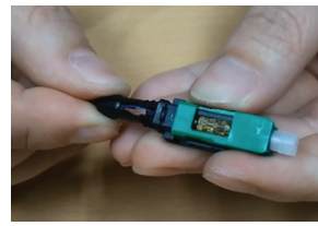
Insert the fiber into the connector body until the strand meets resistance and bows slightly
