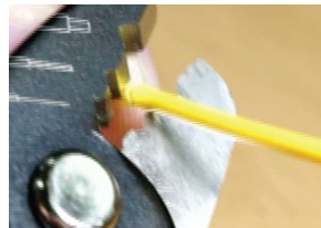
Strip outer jacket about 50mm to reveal 900-micron fibers
