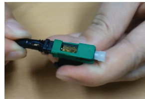
To remove or re-terminate the connector, simply unscrew the boot and replace the jig
