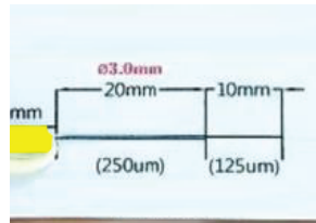
Measure from the end of the jacket and make a mark between the 250µm and 125µm section
