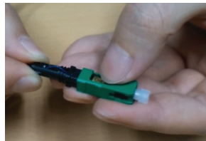
Lock the fiber inside the connector by pressing the amber button
