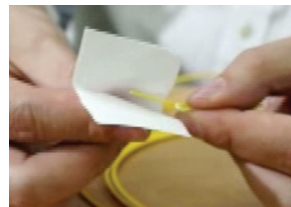
Clean any impurities from your cable using alcohol and a lint-free cloth
