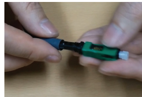
Slide the adapter tube into the connector, then screw the boot onto the connector body and trim any exposed Kevlar yarn
