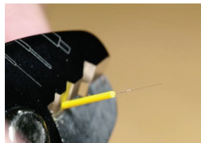
Strip the remaining 20mm of buffer from the edge of the jacket using the middle hole on the stripper
