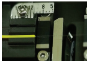
Cleave your fiber strand to 10mm from the 250µm measurement mark
