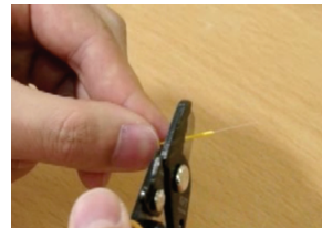
Strip the buffer to the 250µm mark using the middle hole, then the small hole on the stripper in short increments
