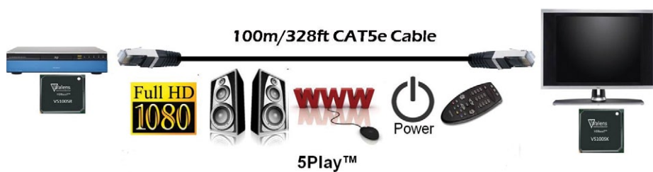
HDBaseT 5Play convergence via a single 100m/328ft Cat5e/6 LAN cable.
