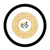
Duplex Plenum Multimode OM3 Fiber Cable is constructed with twelve internal tight buffers, internal aramid yarn, and one outer riser-rated PVC jacket in distribution format. The fiber cable features a water-resistant jacket and is designed for indoor and outdoor applications.
