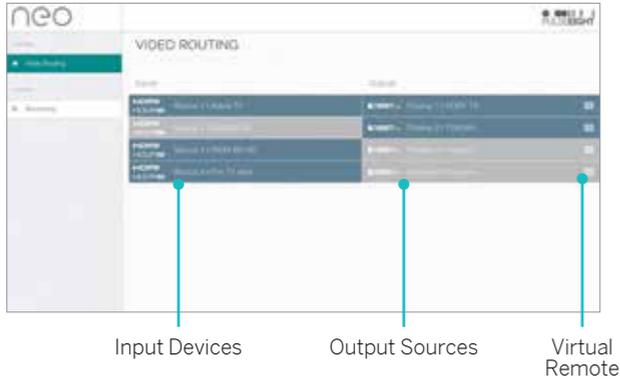
You will see the matrix and the connected input and output devices. This screen is 'drag and drop' to easily change what is displaying on each output.
