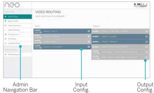
The **Video Routing** tab now gives you the ability to configure your inputs and output including renaming and hiding, plus displaying the status of the connected devices, cable lengths and EDID profiles.
