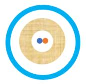
Duplex Riser Multimode OM3 Fiber Cable is constructed with two internal tight buffers, internal aramid yarn, and one outer riser-rated PVC jacket in distribution format. The fiber cable is designed for indoor applications and features Corning ClearCurve fiber.
