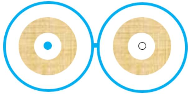
*Duplex Riser Multimode OM3 Fiber Cable* is constructed with two internal tight buffers, internal aramid yarn, and two outer riser-rated PVC jackets in a zip-cord format. The fiber cable is designed for indoor applications and features Corning ClearCurve fiber.
