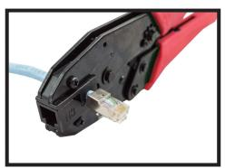
Squeeze the tool to lock the strain relief to hold the cable tightly and grounding
