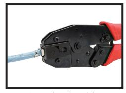
Squeeze the tool to push the contact blades into correct positions
